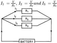
Let  $R_p$  be the resistance of the combination, then  $I = \frac{V}{R_p}$  But  $I = I_1 + I_2 + I_3$
